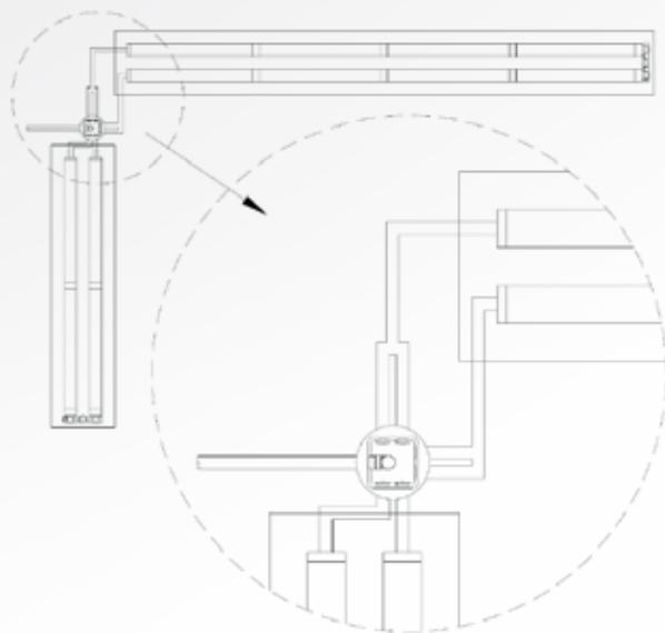
Regarding low-pressure distribution, the number of openings can simply be adapted to the number of pipes per row. For example, for a system with rows of four and rows of two pipes, the rows of four would have twice as many openings as the rows of two pipes. This principle is in fact automatically applied with DBO Expert's low-pressure distribution system (LPDS)!
