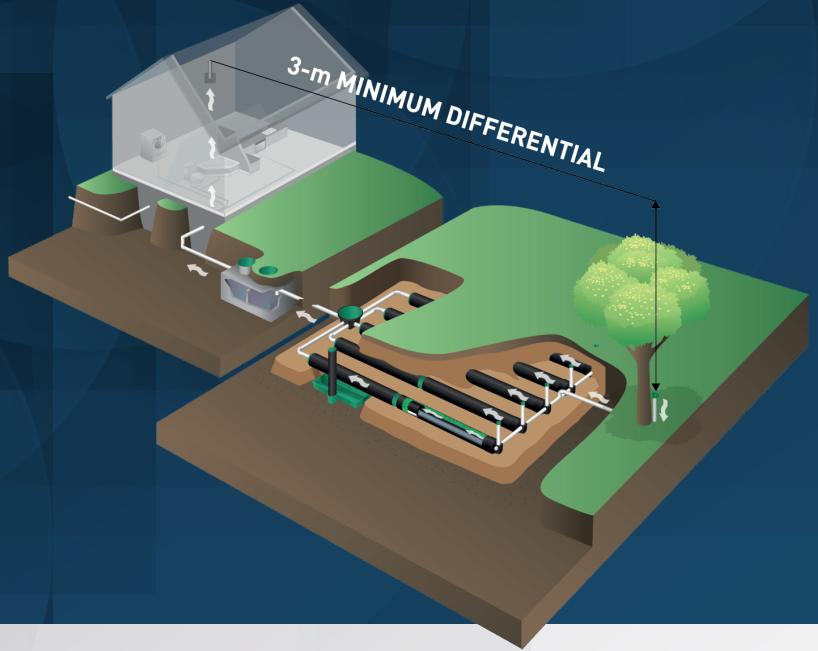
Specific situations can require the ventilation be modified to maintain the proper passage of air.
